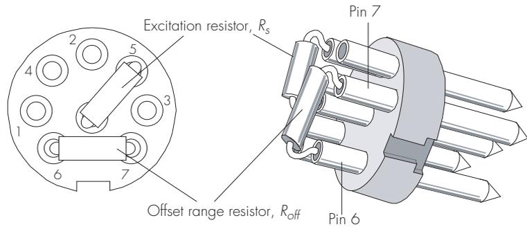
You can zero the signal within the Chart or Scope software, [Figure 2-7](#) and [Figure 2-8](#). This is done by a circuit that uses a 12-bit DAC (digital-to-analog converter) to produce a voltage to zero the signal. The size of this voltage,  $V_{off}$ , is set by a Offset Range Resistor, the value of which,  $R_B$ , is determined by procedures defined below.
