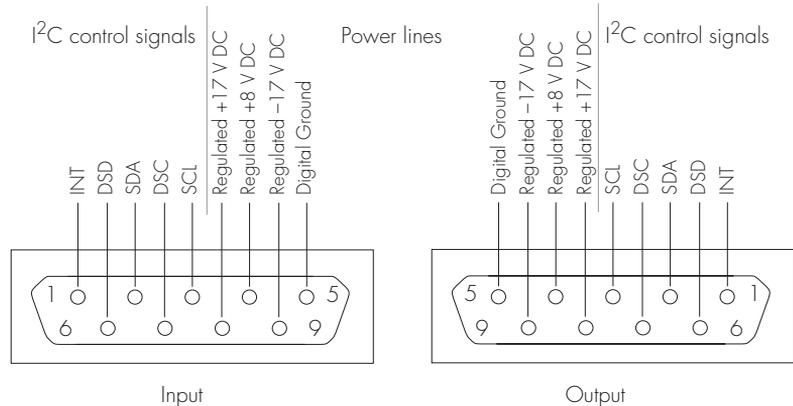
connection to the e-corder (or to the output of other eDAQ Amps). A cable is provided with the Bridge Amp for this purpose. This connection provides power to the Bridge Amp and carries the various control signals (for gain range and filter selection) to and from the e-corder. The pin assignments are shown in [Figure 2-4](#).
