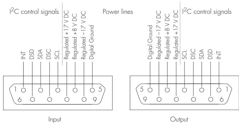
cable is provided with the GP Amp for this purpose. This connection provides power to the GP Amp and carries the various control signals (for gain range and filter selection) to and from the e-corder. The pin assignments are shown in [Figure 3–4](#).
