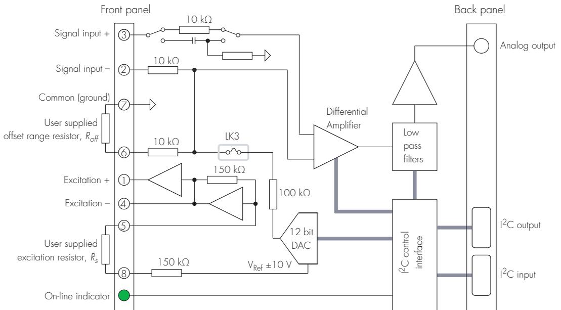
voltage. Signal offsets are zeroed by applying a corrective DC voltage to the negative input stage, under software control. The input amplifier under these circumstances functions as a high impedance single-ended amplifier.
