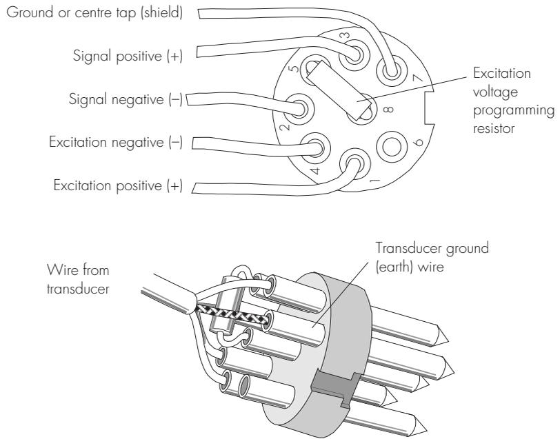
The main insulation sheath of the transducer cable should be clamped with the strain-relief device within the plug. Any unused wires from the transducer should be insulated to prevent shorting of signals or damage to the equipment.
