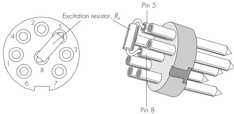
The excitation voltage is set by connecting an Excitation Set Resistor between pins 5 and 8 on the DIN plug of the transducer. Correct mounting of the resistor is shown in [Figure 2-10](#).
